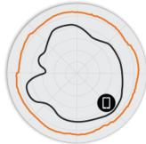
Figure 4. R730 2.4GHz ElevationAntenna Patterns
