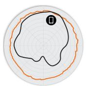
Figure 3. R730 5GHz AzimuthAntenna Patterns
