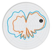
Figure 5. R730 5GHz ElevationAntenna Patterns
